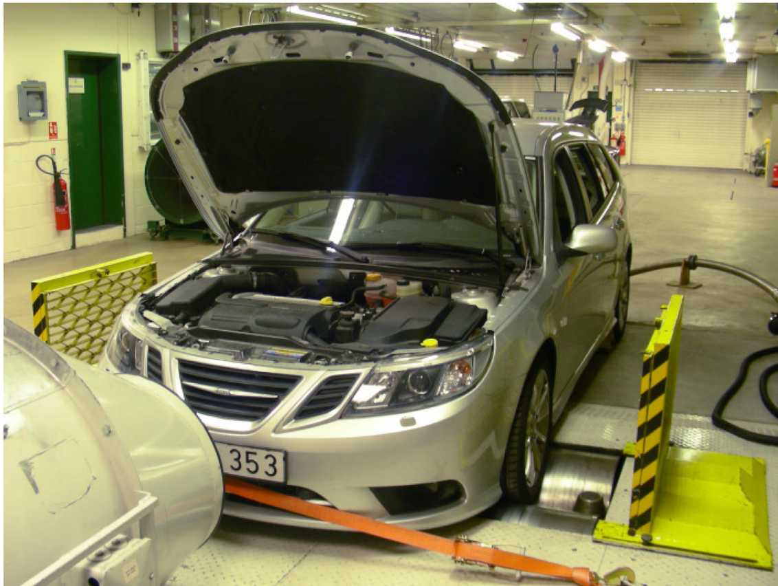
Fig. 2. Photograph of Saab 9-3 BioPower test vehicle on the dynamometer rolls during emissions testing
