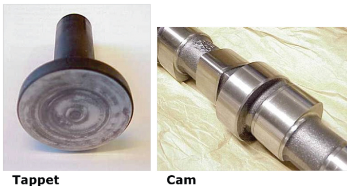
Figure 8. Cummins ISB cam and tappet, low detergent - no ZnDTP, 0.2% ash, 0% phosphorus.
