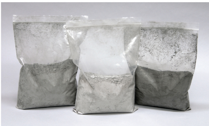
Figure 4. Typical bags of incombustibles received from the Volvo Truck test after each DPF cleaning [6].
