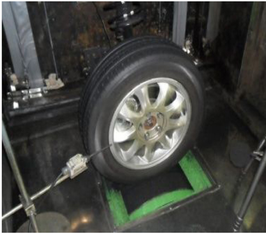
Figure 1. Vehicle setting on 1/4 car dynamometer
