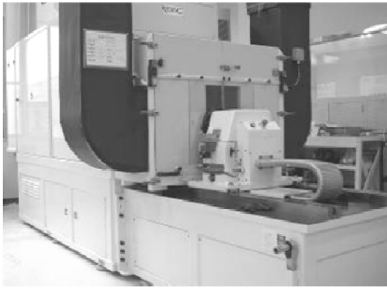
Figure 1. Inertia Dynamometer for measuring dynamic fluid displacement
