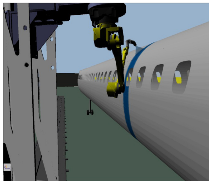
Figure B. Typical Robot/Lift/Rail Configuration
