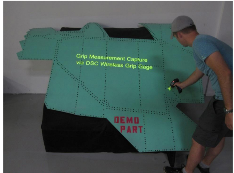
Figure 1. Using a wireless grip gage to measure the highlighted location
