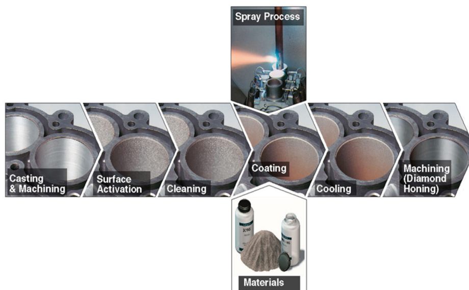
Figure 2. Schematic representation of the SUMEBore coating process (from left to right, including honing)
