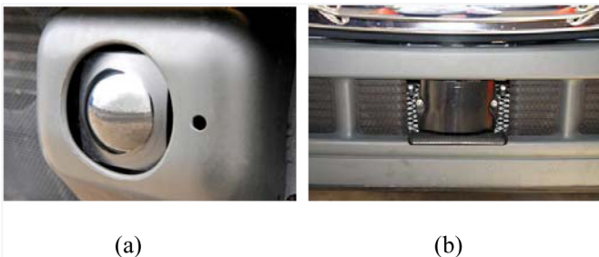
Figure 3. Some of the radar-based FCMS that are available on the market for commercial vehicles include the Bendix Wingman System (a) [11] and the Wabco OnGuard System (b) [12]. Typically these systems are mounted on the front of the commercial vehicle.
