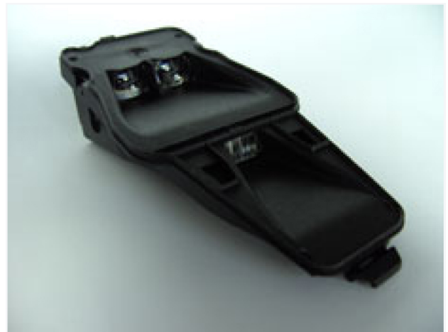
Figure 4. A lidar unit offered in the market as a sensor for active safety systems for passenger cars [18].
