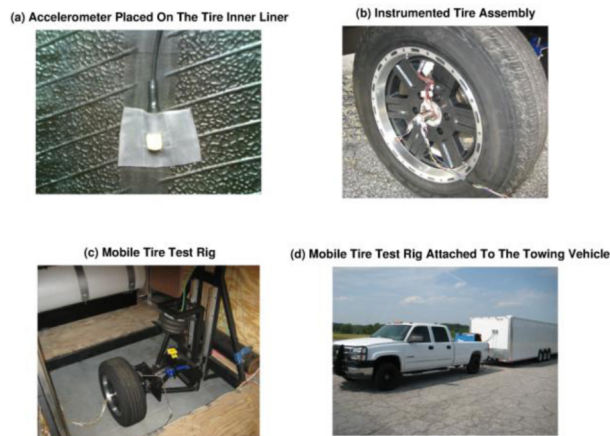
Figure 2. Intelligent tire application: (a) sensor mounting location, (b) instrumented tire assembly, (c) mobile tire test rig, and (d) test rig attached to the towing vehicle
