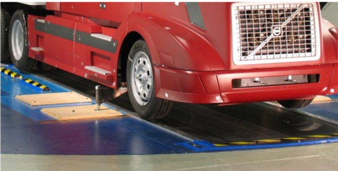
Figure 1. Details of the forward mounts and floor covers.
