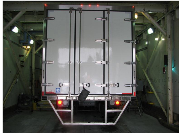
Figure 1. Test vehicle equipped with the control refrigerated box in the environmental chamber (rear view)
