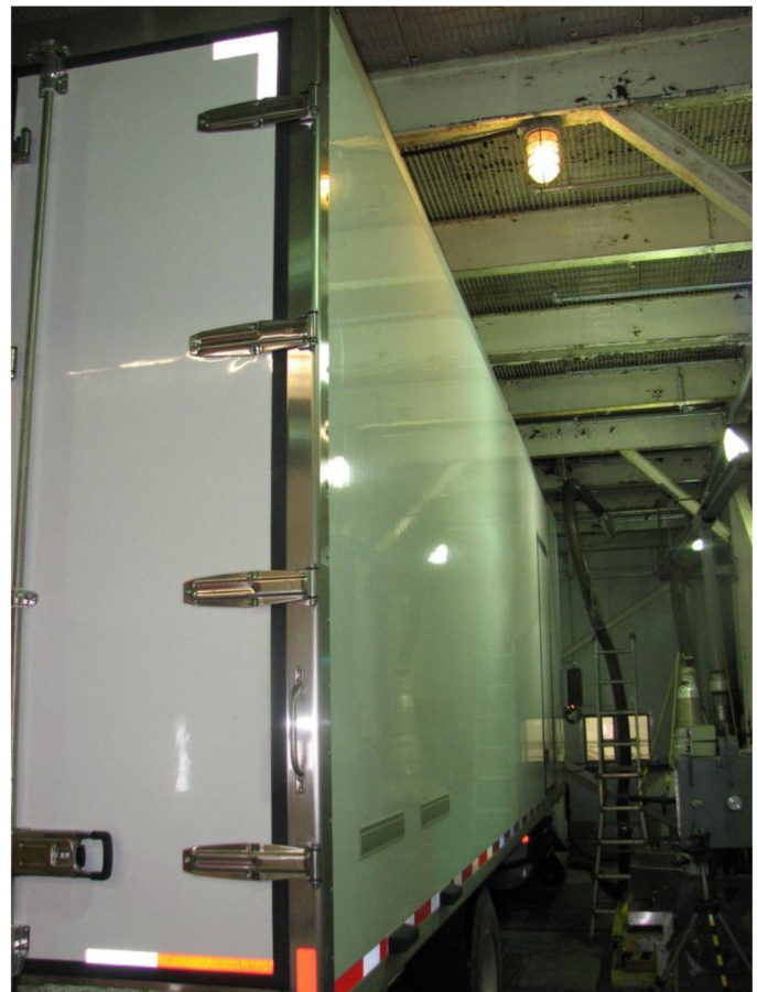
Figure 2. Test vehicle equipped with the test refrigerated box in the environmental chamber (side view)
