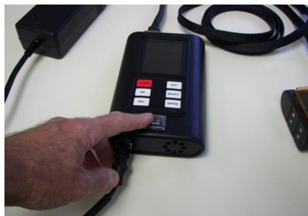
Figure 5. Electronic controller and umbilical cable.
