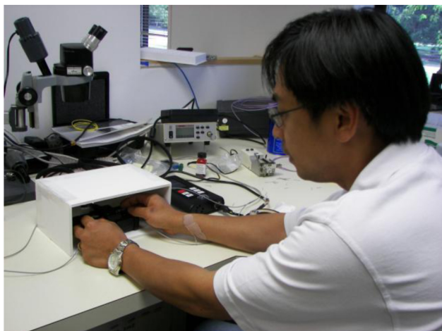
Figure 7. Splicing in a very small cramped space.
