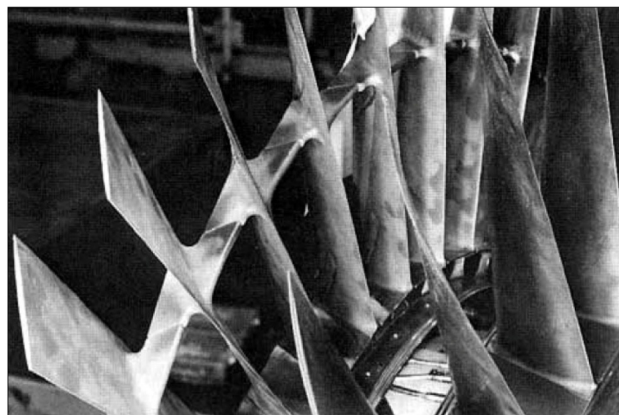
Figure 10. YJ93 first stage titanium compressor blades with midspan shrouds (1960)
