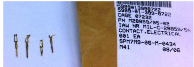
Figure 3. Tuning Fork-type Contact (M28859/5A), Serviceable and Damaged Shown
