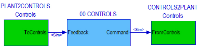
Figure 2. The model that executes on the target Controller during HIL and VDIL phases
