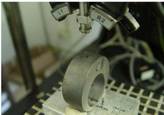
Figure 2. Navy C-Ring ready for residual stress testing
