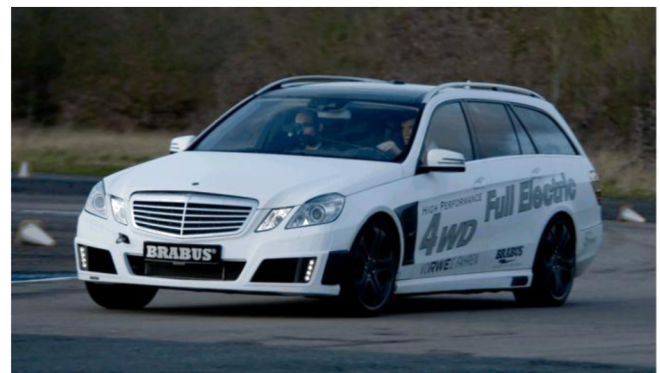
Figure 2. The Brabus 4WD vehicle (EV1) fitted with Protean in-wheel Motors during fault injection testing (Photo D. Harty)
