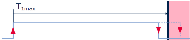
Figure 4. Pulse too long (rising to falling edge)
