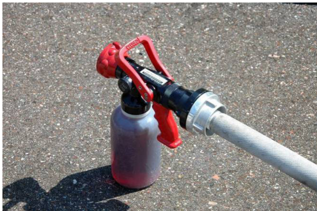
Figure 5. F-500 nozzle used in test 2
