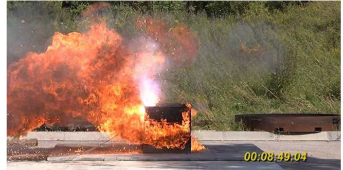
Figure 8. Short circuit inside LiB 1 in minute 8 with the n-heptane still burning
