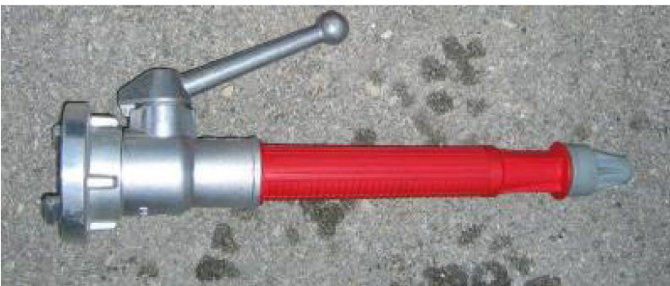
Figure 4. Standardized CM nozzle used in Test 1
