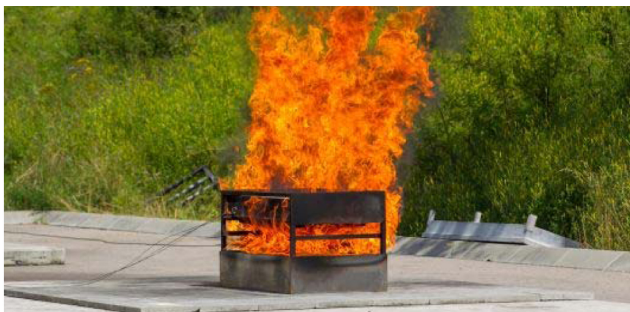
Figure 2. LiB completely surrounded by n-heptane fire to ignite the LiB
