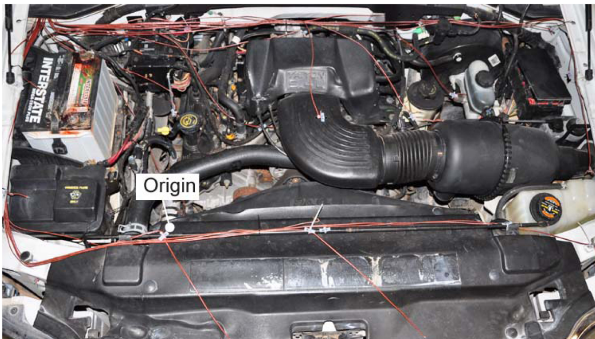
Figure 3. Overview of the engine compartment components, fuel load and the point of origin of the fire.
