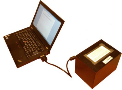
Figure 3. Setup used in the simulations. The external PCI bus is a PCIE4MULTI-EX containing the FPGA card NI PCIe RIO 7852R. The laptop is connected to the bus via an express card.
