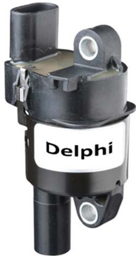
Fig. 4. Remote mount, high energy, Ionization Current enabled ignition coil.
