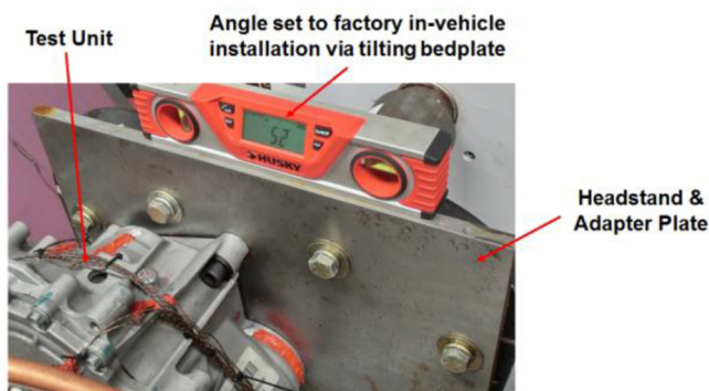
Figure 3. Setting In-Vehicle Installation Angle
