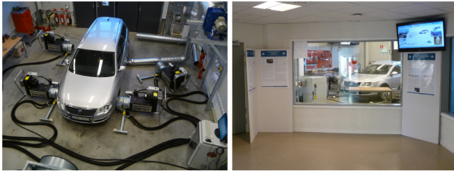
Figure 3. Left: View of the vehicle propulsion laboratory with four mobile dynamometers, head wind fan and exhaust ventilation. Right: View from the corridor.
