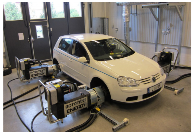
Figure 1. A glance of the new chassis dynamometer lab. A Golf V with a 1.4l multifuel engine has been mounted to the dynamometer units in a 4WD configuration.
