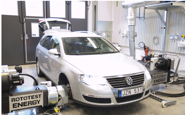
Figure 2. The Volkswagen Passat that is used in the experiment mounted in the chassis dynamometer of the vehicle propulsion laboratory.
