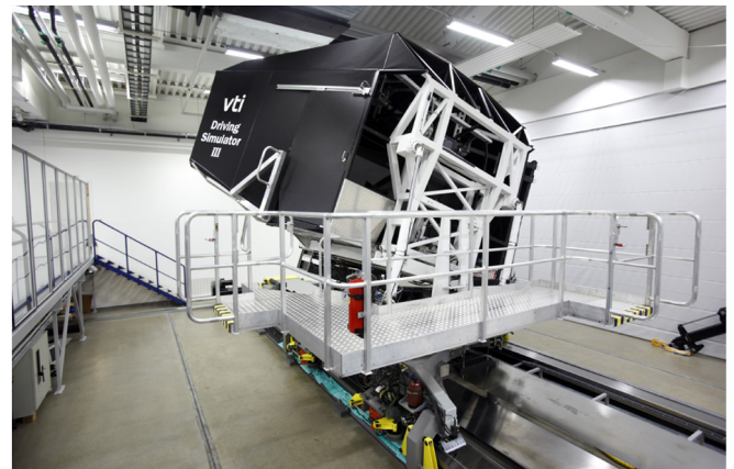
Figure 3. The moving base driving simulator Sim III at VTI.
