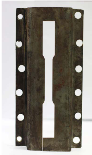
Fig. 5. Formed double-hat face from which a tensile test coupon specimen is extracted
