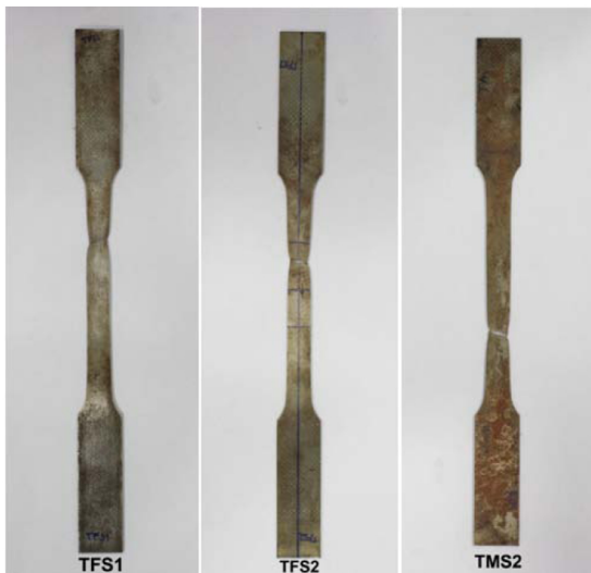
Fig. 6. Tested dog bone shaped specimens
