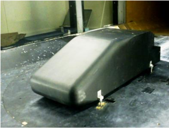
Figure 2. Tapered Windsor Body in the Loughborough University Wind Tunnel
