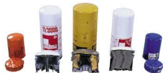
Figure 3. Used oil filters are rarely crushed, but even then they still retain significant amounts of contaminated motor oil.
