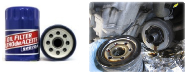
Figure 1. A conventional spin-on, throw-way automotive oil filter and its engine application.
