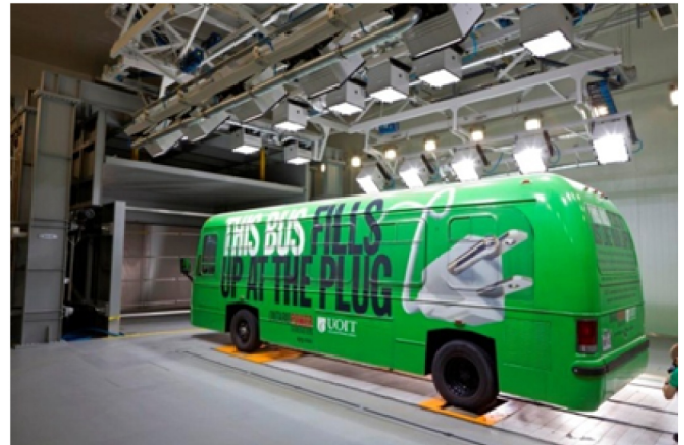
Figure 5. CWT test section configured for icing and solar simulation with 20 \text{ m}^2 nozzle for a large vehicle
