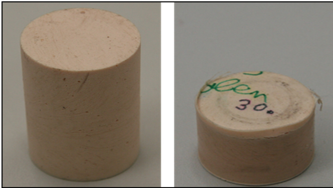
Fig. 8. Test sample ( L=50\text{mm} ), before and after test
