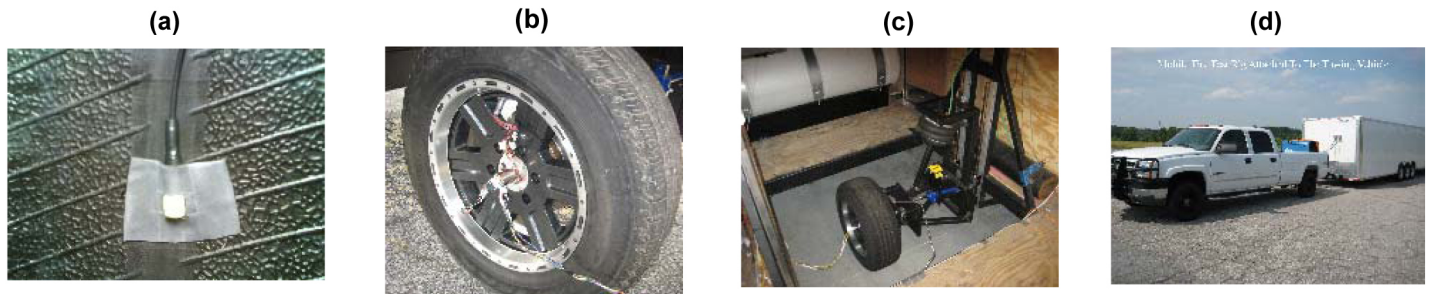
Figure 1. (a) Accelerometer placed on the tire inner-liner (b) Instrumented tire assembly (c) Mobile tire test rig (d) In-house tire testing trailer at the ITL facilities
