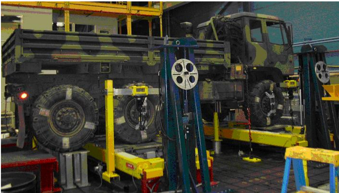
Figure 1. A 3-axle truck being tested on the SPIDER. For this test, only Axle 1 is being tested on the front axle frame. Vehicle Axle 2 is inactive on the rear axle frame.
