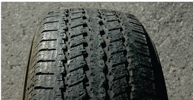
Figure 4. ‘Shaved’ Tire Used in Testing
