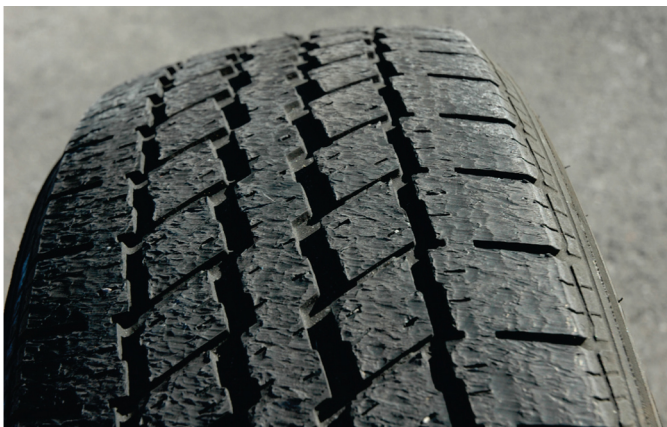
Figure 5. Close-up Photograph of “Shaved” Tire
