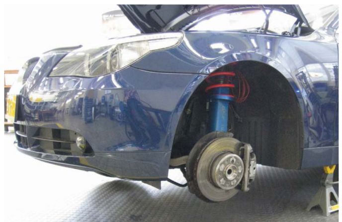
Figure 2. Close-up view of the active suspension system installed on the BMW test vehicle [6, 8].
