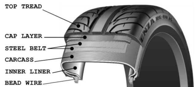
Figure 1. Modern belted radial construction
