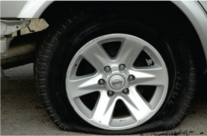
Figure 7. Right Rear Tire After Air Out Event
