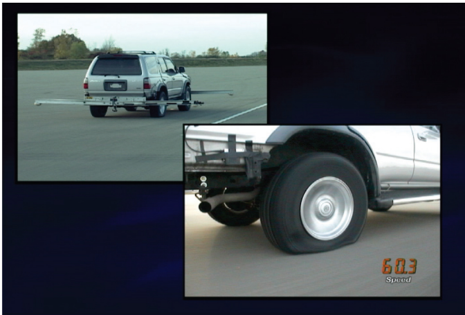
Figure 13. 2000 Compact SUV w/ Deflated Right Rear Tire
