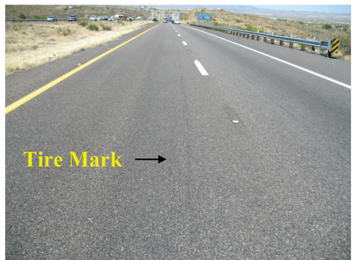
Figure 3. Start of Tire Mark from Right Rear Deflated Tire
