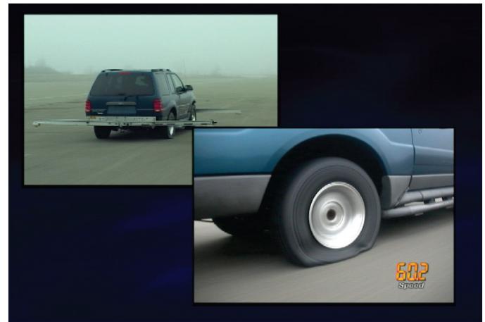
Figure 14. 2001 Compact SUV w/ Deflated Right Rear Tire
