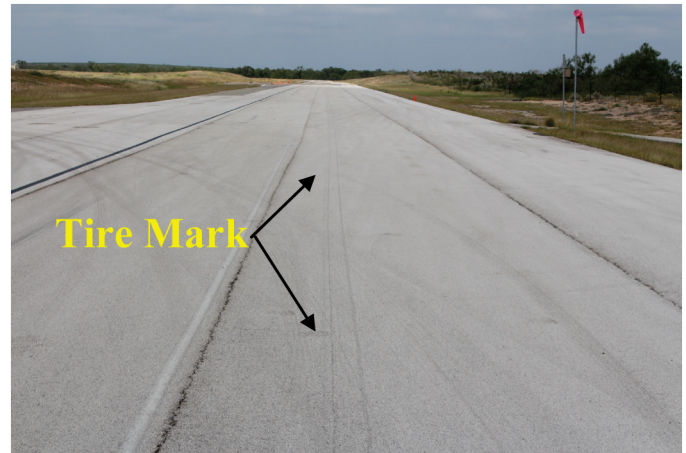
Figure 2. Deflated Tire Mark from 2002 Compact SUV
