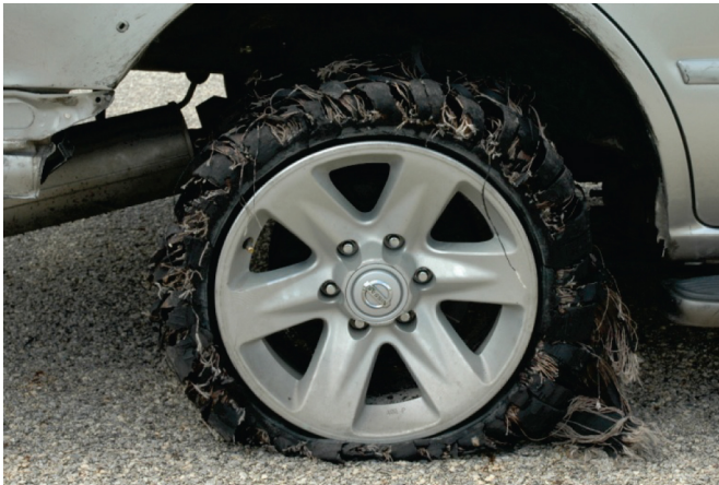
Figure 8. Right Rear Tire After Being Driven Deflated
