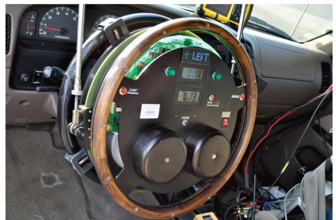
Figure 11. Automated Steering Controller, 2000 SUV Testing
