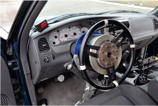
Figure 12. Automated Steering Controller, 2001 SUV Testing
