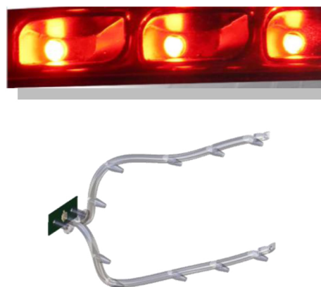
Figure 4. The “light engine” acts as many LEDs
