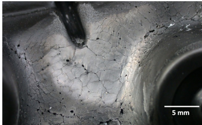
Figure 3. Image of heat check cracking on the surface of a die.
