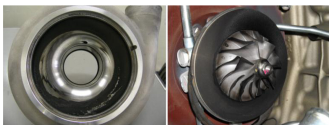
Figure 2. Oil buildup on the compressor's stationary and rotating walls.
