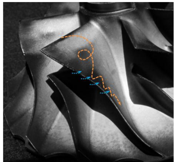
Figure 8. A sketch showing the likely secondary flow field effects contributing to oil deposits within compressor A, operating at high incidence.
