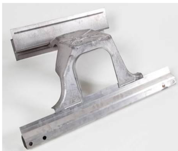
Figure 2. Actual friction-stir welded version of the magnesium-intensive front-end ‘demonstration’ structure less the steel corrosion test plate shown in Fig. 1 .
