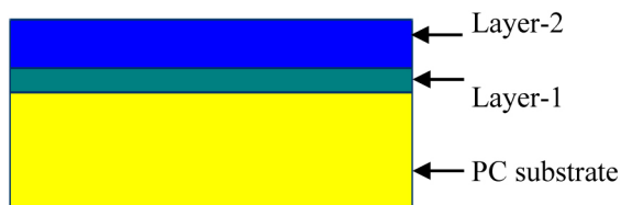
Figure 1. Schematic of a typical two-layer coating system.
