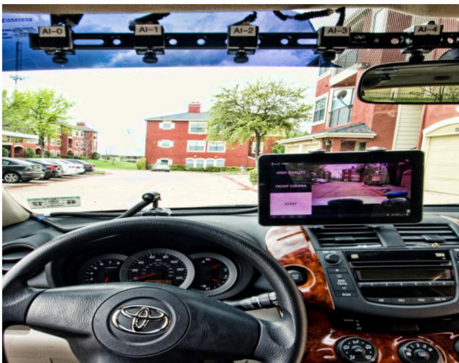
Figure 2. Inside UTDrive data collection vehicle along with the portable device mounted on the windshield.
