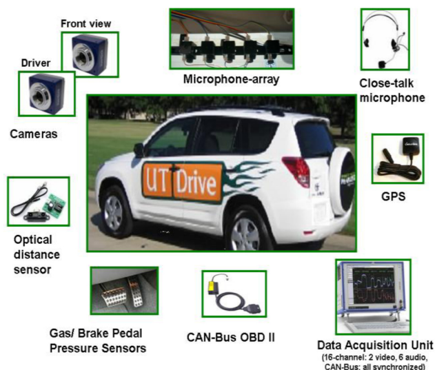
Figure 1. Instrumented UTDive Data collection vehicle along with all the sensors.
