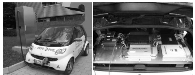
Figure 6. E-Smart experimental BEV (left) and its control system (right)
