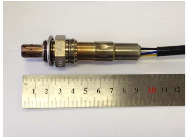
Figure 4. Zirconia AFR sensor
