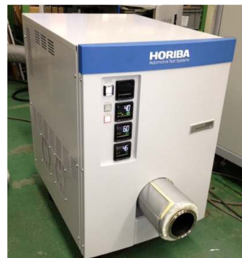
Figure 2. Ultrasonic exhaust gas flow meter
