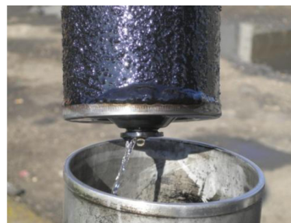
Figure 2. Filter clogging due to microbial activity in the fuel
