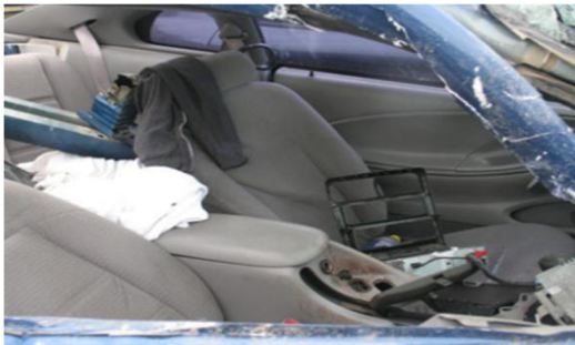
Figure 7. Example of Torso to Center Console Contact in a Far Side Belted Single Occupant Impact, NASS-CDS Case - Rigid Console
