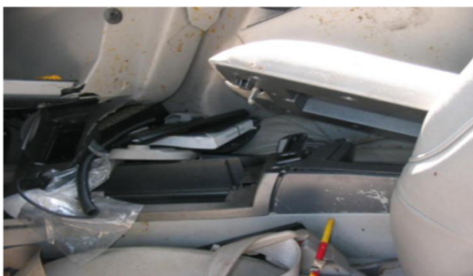
Figure 8. Example of Torso to Center Console Contact in a Far Side Belted Single Occupant Impact, NASS-CDS Case - Deformed Console (Forward in Vehicle is to the Left)
