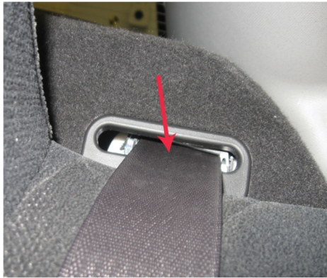
Figure 5. Point recorded on upper anchorages that were not on a pivoting D-ring or did not have an accessible bolt
