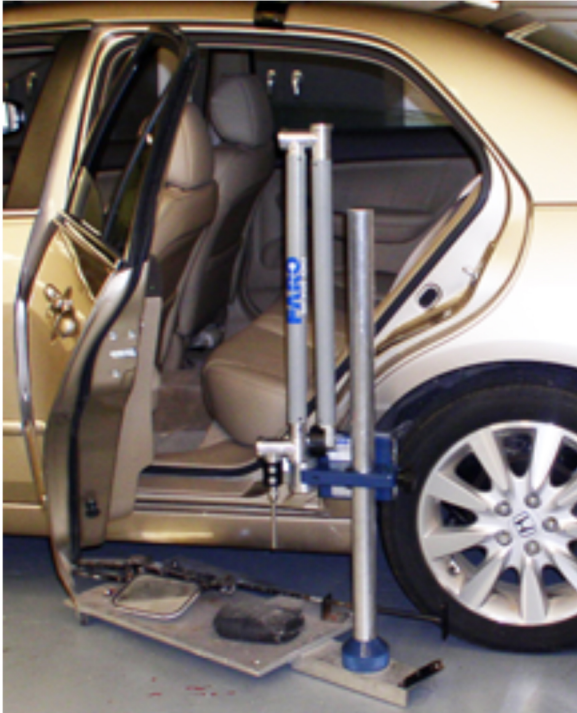
Figure 1. CMM (FARO Arm) attached to a vehicle.
