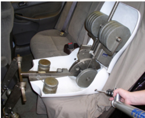
Figure 2. Using CMM to measure seat H-point.
