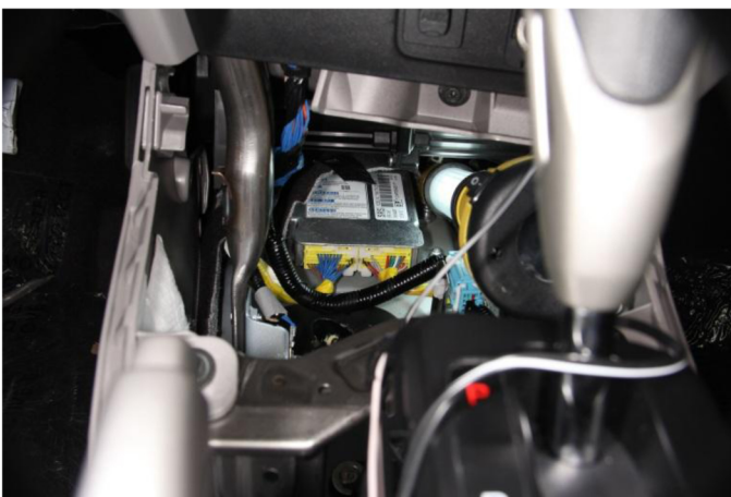
Figure 2. SRS module in the 2012 Civic located in the fore section of the center tunnel.
