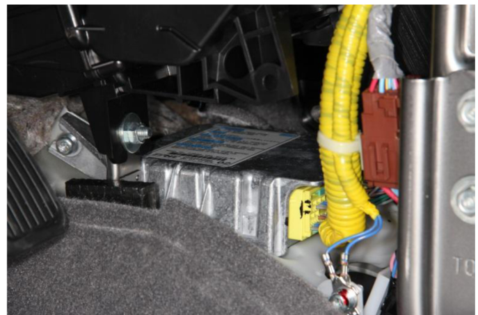
Figure 4. SRS module located to the right of the accelerator pedal in the CR-V.
