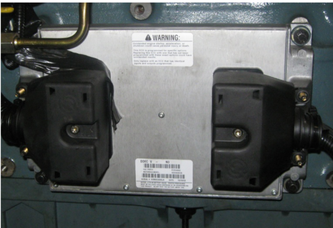
Figure 1. Sample Detroit Diesel DDEC V ECM
