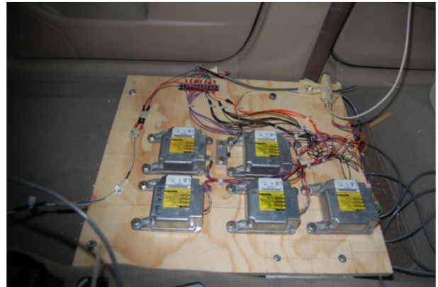
Figure 1. ACM test setup for the in vehicle tests
